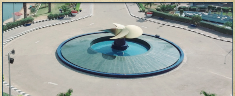
PNS MOAWIN's Propeller on display at the PMM Type - True Screw solid manganese Bronze Number of Blades - 4, Diameter - 14'-6", Pitch - 16' 3"
